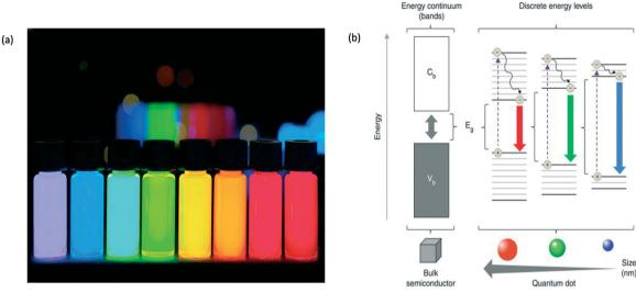
Fig. 1 (a) The different colours that QDs give rise to according to the energy emitted by the crystal; (b) the colour and size of the QD based on the energy level properties.3,16
