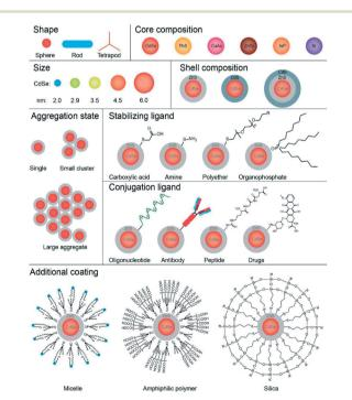
Fig. 2 The different components/shapes of those components in QDs which generate different QDs. Due to the number of different components, it means that they differ in shape/size/properties.<sup>20</sup>
