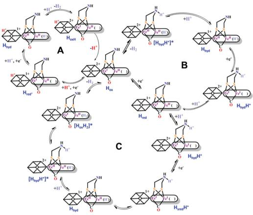
Scheme 22 Proposed catalytic cycles for reversible H<sup>+</sup> reduction by [FeFe]-hydrogenases.<sup>387–390</sup>
