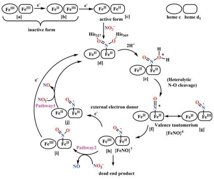
Scheme 20 Proposed reaction mechanism of Cd<sub>1</sub>NiR.
