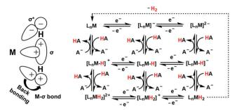
Scheme 25 Schematic presentation of the formation of M-H $_2$   $\sigma$  bond and  $M_{d\pi} \rightarrow H_2$  backdonation (left). Possible mechanistic pathways for catalytic reduction of proton to hydrogen in the natural hydrogenases or synthetic catalysts (right).
