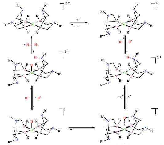
Scheme 35  $H_2$  oxidation (counter-clockwise) and evolution (clockwise) cycle mediated by  $[Ni(P^R_2N^{R'}_2)_2]^{2+}$  molecular catalysts. <sup>548</sup> This cycle is a simplification that neglects certain side reaction pathways, and the order of the steps depends on the identities of substituents R and R'. 428
