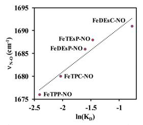
Fig. 21 Correlation between experimentally measured N-O stretching frequency and NO dissociation constant in model complexes.
