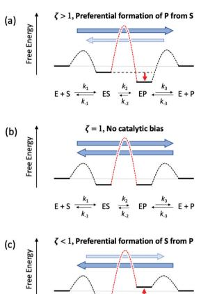
Fig. 1 Schematic representation of an ideal three-stage process for the equiergic interconversion of S and P (the equilibrium constant for  $S \Leftrightarrow P$  is 1, i.e., no thermodynamic driving force in a specific direction) by a catalyst E. Under steady state conditions, if ES
