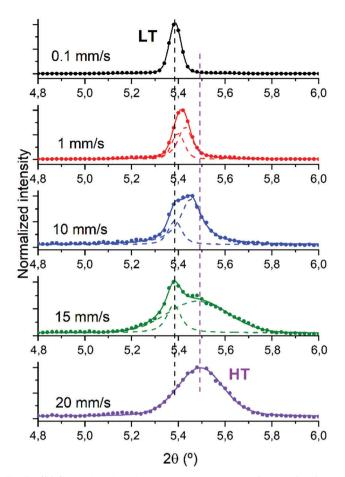
Fig. 3 (001) peak fits of the films fabricated with diF-TES-ADT:PS at 0.1, 1, 10, 15 and 20 mm  $s^{-1}$
