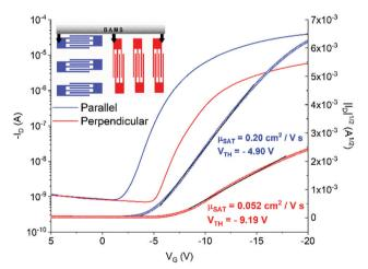
Fig. 5 Transfer characteristics of representative OFET devices with channel length parallel (blue line) and perpendicular (red line) with respect to the solution shearing direction, fabricated at  $1 \text{ mm s}^{-1}$ .
