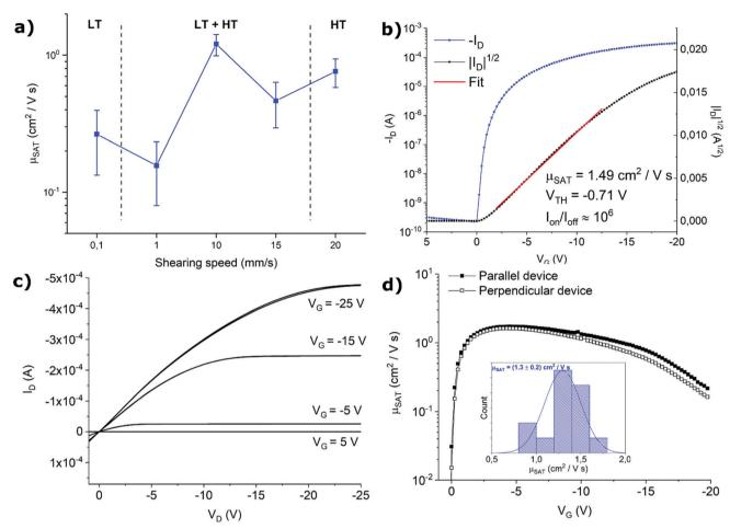
Fig. 4 (a) Mobility vs. shearing speed plot. Representative transfer (b) and output (c) characteristics for a diF-TES-ADT:PS film deposited at 10 mm s<sup>-1</sup>. (d) Mobility profiles for films coated with the channel parallel (filled squares) and perpendicular (empty squares) to the shearing direction (inset: device mobility statistics).
