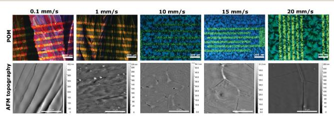
Fig. 2 POM (top panels) and AFM topography (bottom panels) images of the diF-TES-ADT:PS thin film OFETs prepared at different solution shearing speeds. In all these films the shearing directions coincides with the channel length. The scale bars in the AFM images correspond to 10 µm.
