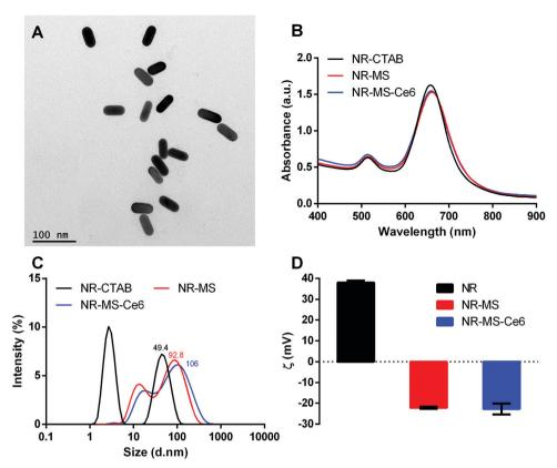
Fig. 2 Characterization of NR-MS-Ce6 and the controls of as-synthesized NR-CTAB and NR-MS showing (A) the monodispersity of the synthesized NR-CTAB used in this study using TEM with  $200\,000\times$  magnification, (B) the UV-vis spectrum, (C) histogram distribution of hydrodynamic diameter ( $D_H$ ) as determined by dynamic light scattering (DLS), and (D) zeta potential of all three samples. Error bars represent standard error for N=3 samples.
