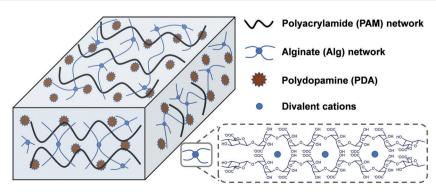
Scheme 1 Schematic structure of PAM-Alg-PDA hydrogel adhesive.
