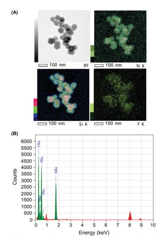
Fig. 6 (A) Bright field (BF) and elemental mapping (Si, N and F) and (B) EDX spectrum of NP3CPT by EDX-TEM.
