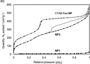
Fig. 5 Solid state <sup>29</sup>Si NMR spectra of **NP** (A) and **NP1** (B). (C) Isotherms of CTAB-free NP, NP1 and NP3 obtained by nitrogen sorption analyses.
