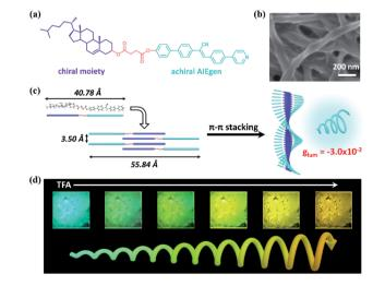
Fig. 1 (a) Chemical structure of Chol-CN-Py. (b) SEM image of xerogel made from DMSO. (c) Proposed molecular packing upon gel formation, leading to blue CPL. (d) Multi-color CPL upon exposure of the xerogel films to different amount of TFA.
