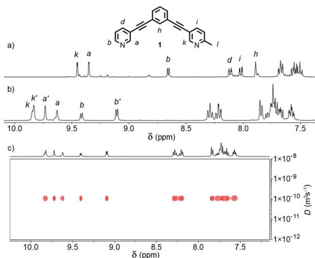
Fig. 2 Partial <sup>1</sup>H NMR spectra (400 MHz, 298 K) of cages [Pd<sub>2</sub>(**1**)<sub>4</sub>](BF<sub>4</sub>)<sub>4</sub> formed in (a) CD<sub>3</sub>CN, and (b) *d*<sub>6</sub>-DMSO; (c) <sup>1</sup>H DOSY NMR spectrum (500 MHz, *d*<sub>6</sub>-DMSO) of *cis*- and *trans*-[Pd<sub>2</sub>(**1**)<sub>4</sub>](BF<sub>4</sub>)<sub>4</sub> cage mixture.
