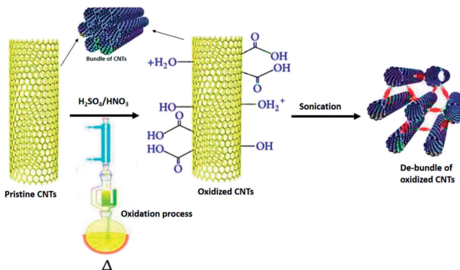
Fig. 6 Functionalisation of CNT through the oxidation process using H 2 SO 4 /HNO 3 . Adapted from ref. 43, copyright 2015, Elsevier.
