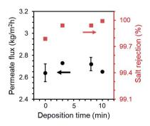
**Fig. 5** Permeate flux and salt rejection of 0.45 μm PP membranes after PHDFA coating with varying deposition time. Test condition: feed temperature at 50 °C, flow rate at 0.81 L min $^{-1}$ , NaCl concentration at 30 g L $^{-1}$ .
