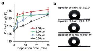
Fig. 3 (a) Effect of vapor deposition time on the wettability of PP membranes with varying pore sizes. (b) Optical images of water droplet on 2  $\mu$ m PP membranes with different deposition time.
