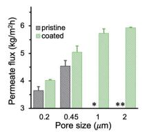
Fig. 7 Permeate flux of PP membranes before and after 8 min of PHDFA coating using high-salinity feed with 100 g L $^{-1}$  NaCl. The pristine 1 and 2  $\mu m$  membranes leaked during MD while the coated membranes remained nonwetted. \* and \*\* indicate intermittent and frequent leaking, respectively.
