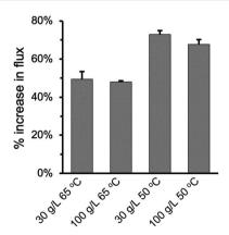
Fig. 8 Percentage increase in the permeate flux under different operation conditions when the nominal pore size increases from 0.2  $\mu$ m to 2  $\mu$ m for PP membranes after 8 min of PHDFA coating.
