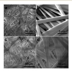
Fig. 2 SEM images of 2  $\mu$ m PP membranes before (a and b) and after (c and d) 8 min chemical vapor deposition of PHDFA.
