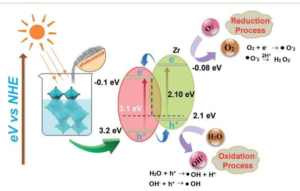
Fig. 2 Photocatalytic mechanism of dye degradation in the presence of Zr-TiO<sub>2</sub> photocatalyst.
