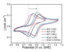
Fig. 1 CV curves of five TEMPO derivatives (1 mM) in 0.5 M KCl supporting electrolyte (pH = 7) at a scan rate of 25 mV s $^{-1}$  at 25 °C. Before CV measurements, the pH values of the electrolyte solutions were adjusted to 7 for 4AT and 4CaT by using 0.01 M HCl and KOH solution, respectively, because 4AT is weakly alkaline and 4CaT is weakly acidic.
