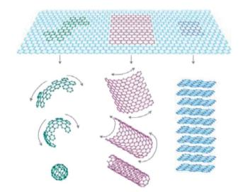
Fig. 1 Carbon allotropes: graphene to fullerene, nanotubes and graphite. This figure has been reproduced from ref. 19 with permission from Springer Nature, Copyright 2007.
