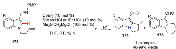
Scheme 42 Intramolecular hydroarylation leading to dihydropyrrolo-indole and tetrahydropyridindole.
