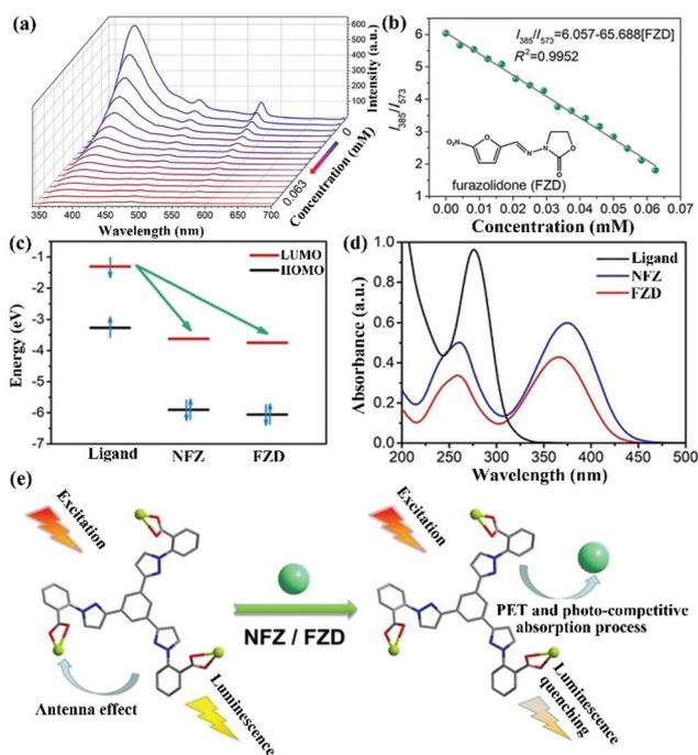
**Fig. 10** (a) The emission intensity and (b) fitting curve of Dy-TCPB upon incremental addition of FZD. (c) The electron transfer from the LUMO of the ligand to the LUMO of NFZ or FZD. (d) The absorption band of H<sub>3</sub>TCPB and NFZ/FZD. (e) The sensing mechanism of Dy-TCPB toward NFZ/FZD. Reproduced from ref. 103 with permission from Wiley-VCH.
