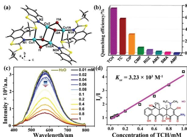
**Fig. 6** (a) The crystal structure of UJN-Cu2. (b) Quenching efficiencies of NJU-Cu2 toward different antibiotics. (c) Luminescence spectra of NJU-Cu2 in TCH aqueous solutions in the concentration range of 0–1.0 mM. (d) Stern–Volmer plots of UJN-Cu2 toward TCH. Reproduced from ref. 85 with permission from the American Chemical Society.
