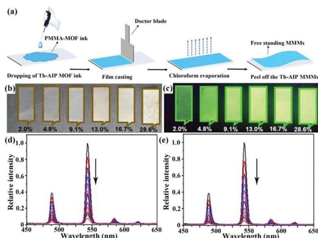
**Fig. 23** (a) The preparation process of Tb-AIP MMMs. Images of Tb-AIP MMMs by varying the additional amounts of MOF powders (b) under natural light and (c) UV lamp at 365 nm. Emission spectra of Tb-AIP MMMs upon increasing concentrations of (d) NFZ and (e) NFT. Reproduced from ref. 127 with permission from Elsevier.
