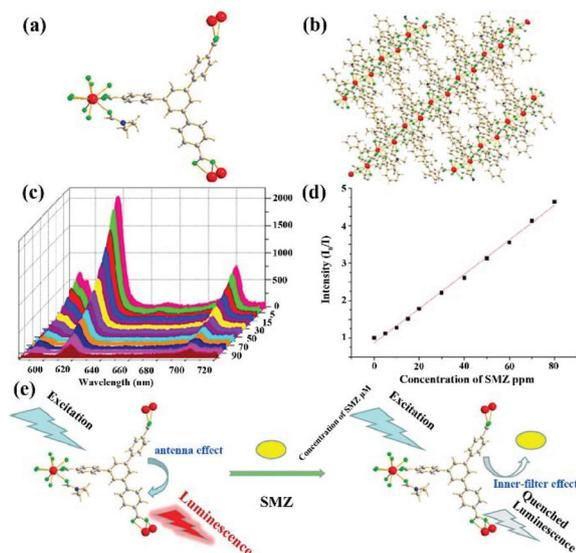
**Fig. 7** (a, b) The structure of Eu-MOF. (c) Emission spectra of Eu-MOF at different SMZ concentrations. (d) Stern–Volmer plots of  $I_0/I$  and SMZ concentrations. (e) A possible mechanism of the inner filter effect for SMZ detection. Reproduced from ref. 92 with permission from the American Chemical Society.
