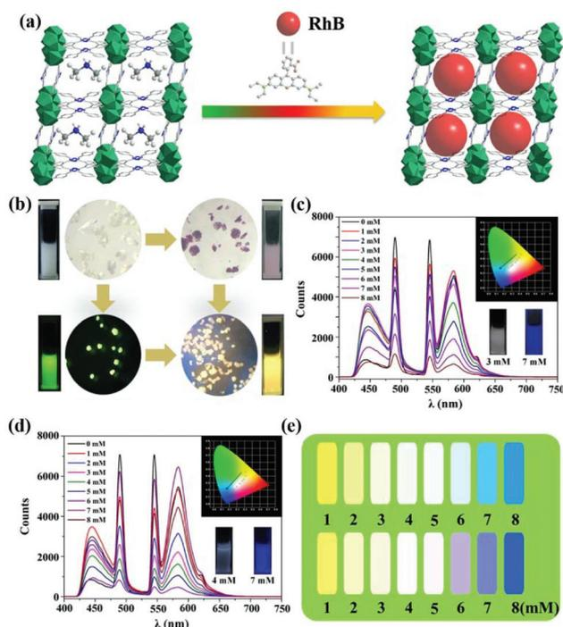
**Fig. 16** (a) The 3D porous anion framework of Tb-dcpct and the fabrication of RhB@Tb-dcpct via cation exchange. (b) Photographs of both samples under natural light and UV lamp at 365 nm. Emission spectra of the RhB@Tb-dcpct aqueous suspension upon various concentrations of (c) NFX and (d) CPFY. (e) The corresponding luminescence colours. Reproduced from ref. 117 with permission from the American Chemical Society.
