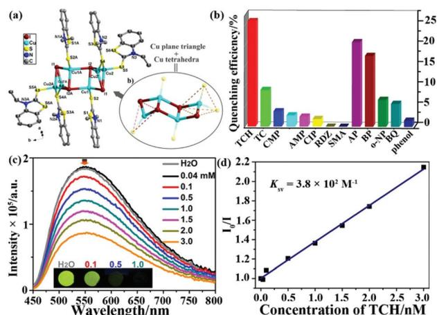
**Fig. 5** (a) The chair-like [Cu<sub>4</sub>I<sub>4</sub>] cluster and whole structure of UJN-Cu. (b) Quenching efficiencies of UJN-Cu toward different antibiotics. (c) Emission peaks of UJN-Cu in aqueous solutions with increasing TCH concentration. (d) The Stern-Volmer relationship of I<sub>0</sub>/I and TCH concentration. Reproduced from ref. 84 with permission from the American Chemical Society.
