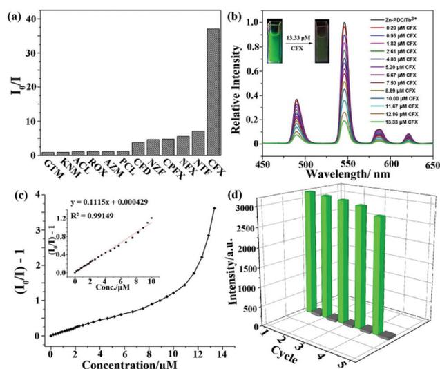
Fig. 12 (a) Luminescence quenching efficiencies of Zn-PDC/Tb<sup>3+</sup> at 546 nm toward different antibiotics. (b) Emission peaks, (c) Stern-Volmer plots and (d) the reusability of Zn-PDC/Tb<sup>3+</sup> toward CFX. Reproduced from ref. 111 with permission from the American Chemical Society.
