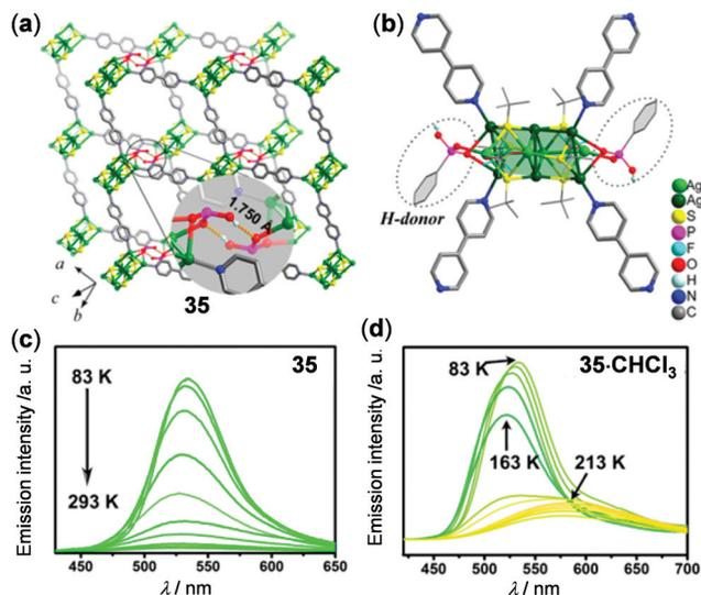
**Fig. 29** (a) Two-layer stack and (b) perspective view of the coordination environment of Ag-MOF **35**. (c and d) Temperature-dependent solid-state emission spectral change of (c) **35** and (d) **35-CHCl<sub>3</sub>**. Reprinted with permission from ref. 131. Copyright 2018 American Chemical Society.
