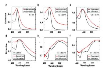
Fig. 10 Extinction spectra of isolated Au nanocrystals and assemblies of various sizes. (a)  $5.5 \pm 0.4$  nm Au nanocrystals; Au aggregates with sizes of (b) 52  $\pm$  22 nm, (c) 125  $\pm$  25 nm, and (d) 198  $\pm$  84 nm; Au supracrystals with sizes of (e) 413  $\pm$  128 nm and (f) 611  $\pm$  138 nm. The average sizes were used to fit the measured data.
