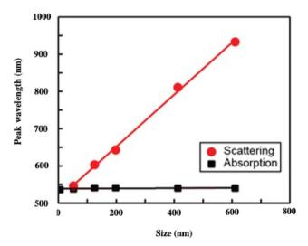
Fig. 11 Variation of the peak wavelength as a function of the assembly size: the black curve illustrates the absorption peak of Au that is present for all assemblies. The scattering peak represented in the red curve red shifts as the assembly size increases.
