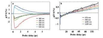
Fig. 14 Dynamics of  $\Delta T/T$  at selected probe wavelengths, at the two different time scales of energy flow in the Au clustered structures (a and b). From these data, a water dispersed Au "clustered" structure can be operated as very efficient nanoheaters whereas it was not observed in dried Au supracrystals.
