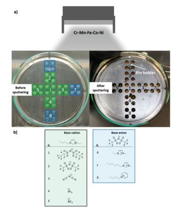
Fig. 1 (a) Schematic of sputtering into a library of 8 ILs to obtain a library of CSSNPs. From the Cr-Mn-Fe-Co-Ni alloy target atoms are sputtered simultaneously and deposit in different ILs contained in a cavity holder. Photographs before and after sputtering show a color change after sputter synthesis in the ILs. (b) Molecular structures of the 8 ILs divided in two subgroups according on the common cation and
