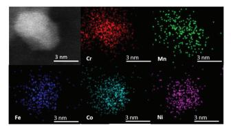
Fig. 4 STEM high angle annular dark field image and corresponding EDS elemental mapping from the CSSNPs synthesized in IL 8. All elements are homogenously distributed.
