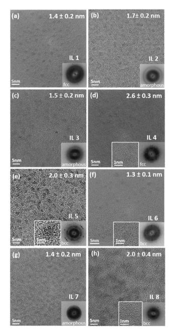
Fig. 3 HRTEM images of CSSNPs sputtered in 8 different ILs: (a) IL 1, (b) IL 2, (c) IL 3, (d) IL 4, (e) IL 5, (f) IL 6, (g) IL 7 and (h) IL 8. The insets show the zoom in on the crystalline CSSNPs and the FFT patterns with the deduced crystal structure. Amorphous, fcc or bcc CSSNPs were found depending on the IL used in the synthesis.
