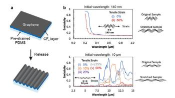
Fig. 3 Conformal graphene wrinkles for tunable emissivity. (a) Scheme describing conformal wrinkling of graphene on fluoropolymercoated PDMS. (b) Emissivity of nanotextured graphene with different feature sizes. Panel a adapted with permission from ref. 55. Copyright 2020 American Chemical Society. Panel b adapted with permission from ref. 70. Copyright 2019 American Chemical Society.
