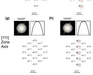
Fig. 2 Simulated images and diffraction patterns for BCC single crystal (left) and twinned NPs (right) from Fig. 1b and c, reproduced in (a and b). (c-h) Projected thickness maps as a proxy for HAADF-STEM images, thickness profile along the yellow line, and simulated diffraction patterns, with parent in black and twin in red. Diffraction spots areas scale with intensity.
