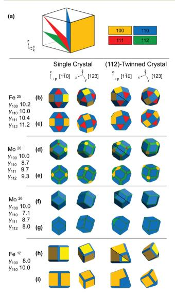
Fig. 1 Shapes of BCC NPs. (a) Dense crystallographic planes in BCC and their color-coding. (b, d, f and h) Analytical thermodynamic and (c, e, g and i) numerical kinetic shapes from the surface energies/growth velocities listed: twin planes are shown as a black line viewing directions are [1 $\bar{1}$ 0] or [123]; these and the x, y, z directions refer to the parent crystal, on, for [110], the bottom left of and, for [123], behind the crystal.
