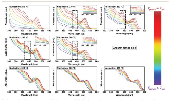
Fig. 1 In situ UV-VIS absorption spectra during the syntheses of CdSe NCs. Each graph contains ten spectra:  $t_{nucl.} = t_{growth}$ , in brown. The spectra in the following colours (to the blue) belong to decreasing growth temperatures, in steps of 10 °C. The growth time in each case is 14 s. Dashed rectangles indicate the presence of MSCs-437.
