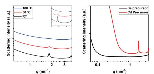
Fig. 3 Left: SAXS patterns of the precursor mixture at different temperatures prior to nucleation. The inset shows a magnification of the Bragg peaks observed above 1 nm<sup>-1</sup>. Right: Scattering curves of the individual Cd and Se precursors.
