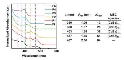
Fig. 4 Absorption spectra for the fraction obtained by size selective precipitation from the reaction mixture at 350 °C and 4.5 s. The table shows the absorption maxima of the CdSe species, their diameters and the calculated aggregation numbers. Fi is the initial sample and F1, ..., F5 the consecutive fractions obtained.
