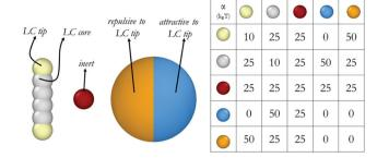
Fig. 1 Molecular models and repulsion parameters implemented for the DPD calculations conducted in this study.
