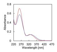
**Fig. 2** Temperature-dependence of the absorption spectrum of hybrid A·B. Conditions: 1  $\mu$ M A·B, 10 mM sodium phosphate buffer pH 7.2, 0.1 mM spermine·4 HCl, 20 vol% ethanol at 75 °C (red) and 20 °C after thermally controlled (0.5 °C min<sup>-1</sup>) assembly process (blue).
