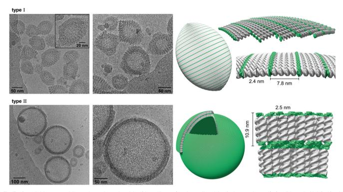
Fig. 3 Cryo-EM images and illustrations of type I vesicles (sheet-like, top) and type II vesicles (columnar, bottom). Conditions:  $1 \mu M \text{ A-B}$ , 10 mM sodium phosphate buffer pH 7.2, 0.1 mM spermine-4 HCl, 20 vol% ethanol.
