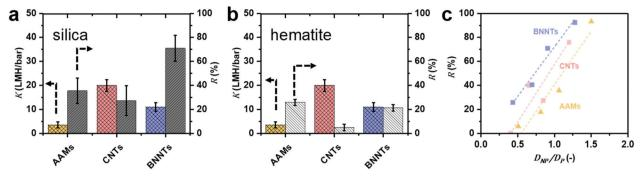
Fig. 4 Experimental permeance K and rejection R for (a) negatively charged silica (pH = 5.5) and (b) positively charged hematite (pH = 5.3) nanoparticles are reported for particles S3, which is smaller than the average CNT and BNNT and comparable with the AAM ( $D_{NP} \le D_P$ ). Full information on the particles and nanotubes, including sizes, can be found in Table 1. (c) Calculated silica NP rejection of AAMs, CNTs and BNNTs membranes as a function of  $D_{NP}/D_{P}$ .
