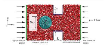
Fig. 2 MD snapshot of case setup for BNNT membrane with particle placed in the solvent reservoir (left); a slice is taken at the xy plane of the domain for a better visual of the system.
