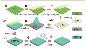
Fig. 1 Schematic fabrication process of grid/wrinkle nanostructures.
