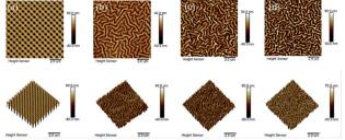
Fig. 2 AFM images of PDMS films with grid nanostructures (a) and wrinkle nanostructures with different etching times: (b) 10 s, (c) 30 s,
