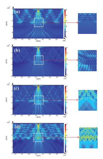
Fig. 6 Calculated distribution of the power near field intensity at the interface between ITO glass and air without (a) and with (b) grid nanostructures at a wavelength of incident polarized light of 526 nm (c) wrinkle nanostructure and (d) multiscale grid/wrinkle nanostructures. Enlargement: detail image of field intensity at the interface between ITO glass and air without and with PDMS nanostructures.
