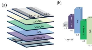
Fig. 1 (a) Device structure and (b) energy level diagram of the QLEDs
