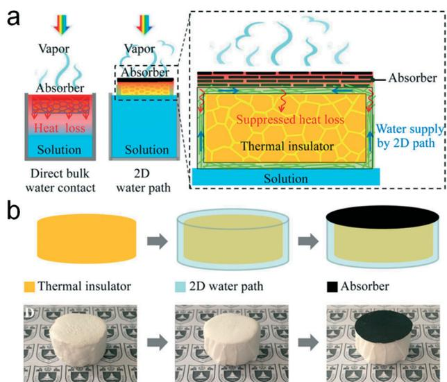
**Fig. 4** Typical evaporator in indirect contact mode.<sup>36</sup> (a) The comparison and the mechanism of the interfacial solar evaporator. The heat loss is strongly suppressed by the insulator, and water can be continuously pumped to the evaporating interface through the 2D path. (b) The rapid fabrication of the evaporator in indirect contact mode.
