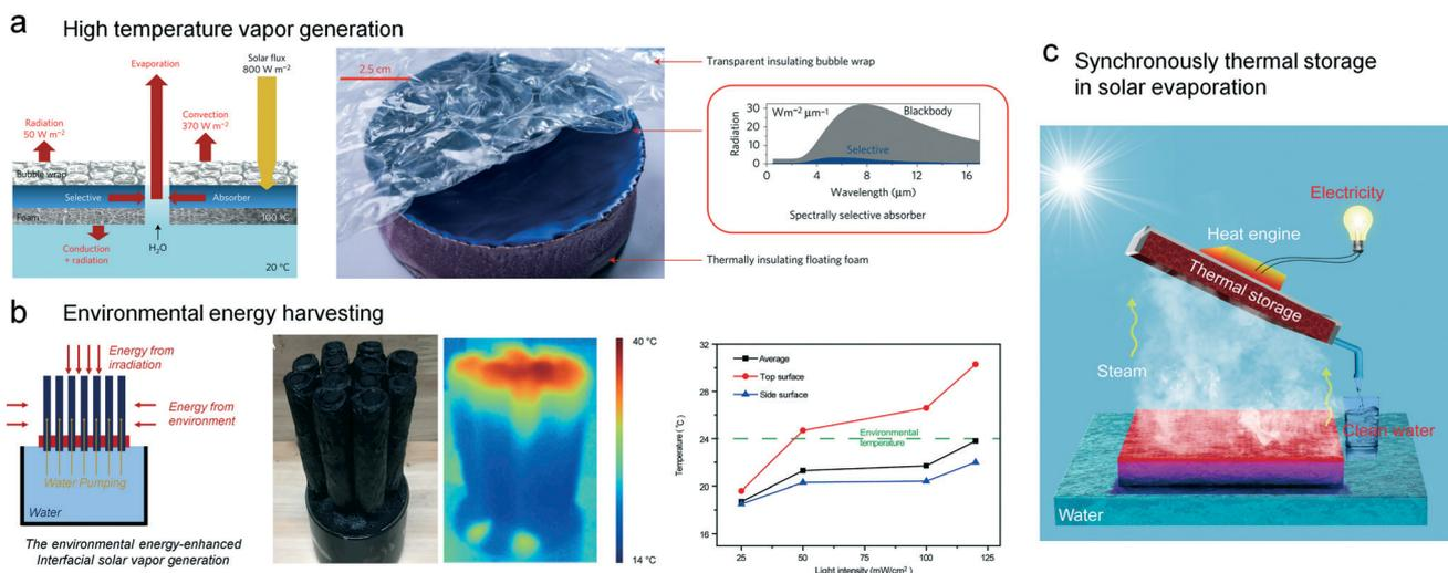
Fig. 10 Innovative solar evaporators with heat managing design. (a) The evaporator with multi-level high insulation for high temperature vapor generation.<sup>59</sup> (b) Smart design for harvesting environmental energy through a wetted side wall. (c) Harnessing the heat of vapor by the water collector for electricity generation.<sup>66</sup>
