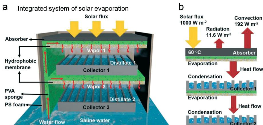
**Fig. 14** The multi-level water production device with integrated evaporation and collection design.<sup>72</sup> (a) The illustration of this solar assisted water production including saline water pumping, vapor generation, and vapor condensation. (b) The heat utilization of this integrated device. The heat flow from the solar irradiation can continuously generate the vapor at different levels.
