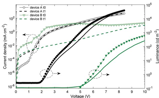
**Fig. 3** *JVL* characteristics of encapsulated top-emitting OLEDs after fabrication (t0) and after seven months (t1). The samples were stored under ambient conditions. Device A has the following stack: glass/Ag/ZnO/TPBi:PEIE/SY/MoO<sub>x</sub>/Ag/MoO<sub>x</sub> with evaporated Ag electrodes. Device B corresponds to the all solution-processed OLED, for which the electrodes are replaced by an ink-jet printed Ag layer on PET and a spin-coated WO<sub>x</sub>/*Clevios F HC* layer.
