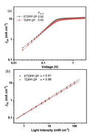
Fig. 3 Plots of photocurrent density  $(J_{ph})$  versus effective voltage  $(V_{eff})$ curve (a), current density ( $J_{sc}$ ) versus light intensity ( $P_{light}$ ) (b) of the **ETDPP-2P** and TDPP-2P devices.
