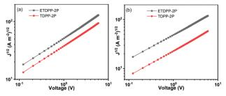
Fig. 4 Dark current-voltage characteristics of (a) hole only device on Glass/ITO/PEDOT: PSS/active layer/MoO<sub>3</sub>/Au and (b) electron only device on glass/Al/active layer/Al under optimized conditions.
