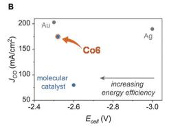
Fig. 12 Comparison of selectivity (A) and activity (B, partial current density) for CO production with **Co6** inserted in a zero-gap membrane flow reactor and previous molecular and heterogeneous CO<sub>2</sub> reduction electrocatalysts (adapted from ref. 118 with permission from AAAS, copyright 2019).
