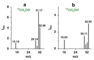
Fig. 15 GC/MS spectra and fragmentation pattern for the electrocatalyzed CO<sub>2</sub> conversion into CH<sub>3</sub>OH. Graphs show the mass fragmentation pattern of CH<sub>3</sub>OH (m/z 29 to 33) produced employing (a) <sup>12</sup>CO<sub>2</sub> or (b) 13CO2 as a reactant substrate. Reproduced with permission from ref. 250
