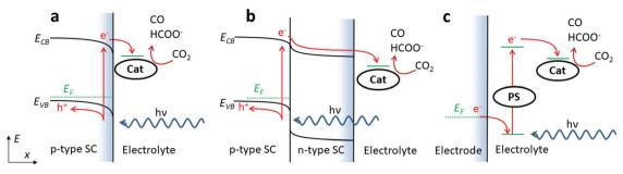
Scheme 5 Possible photoelectrode configurations including molecular catalysts. (a) Catalyst at a p-type photocathode, (b) catalyst at a p-n photocathode, and (c) association between a catalyst and a sensitizer (PS) at a dark electrode surface.
