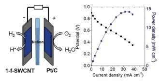
Fig. 11 Polarization (black) and power density (blue) curves for an MEA employing [Ni( $P_c^{\text{Sy}}N_c^{\text{Arg}}$ )<sub>2</sub>]<sup>7+</sup> (denoted as 1-f-SWCNT) and Pt/C as the anode and cathode catalysts, respectively. Experimental conditions: anode loading: 0.3  $\mu$ g cm<sup>-2</sup>, cathode loading (Pt/C): 1 mg cm<sup>-2</sup>, Nafion® as the polymer electrolyte, 60 °C cell temperature. Reprinted with permission from ref. 297. Copyright 2017 Wiley-VCH.
