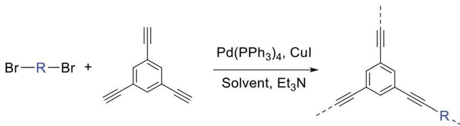
**Fig. 1** The preparation of the CMP networks formed via a palladium-catalysed Sonogashira–Hagihara reaction of 1,3,5-triethynylbenzene with an aromatic DBM.
