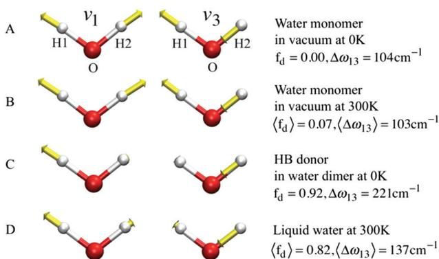
Fig. 11 The symmetric ( $\nu_1$ ) and asymmetric ( $\nu_3$ ) stretching modes of a water molecule and their splitting frequency  $\Delta\omega_{13} = \omega_3 - \omega_1$  in vacuum at 0 K, (B) in vacuum at 300 K, (C) of the H-bond donor of a water dimer at 0 K, and (D) in liquid water at 300 K, respectively. See eqn (7) for the definition of  $f_d$ . Reprinted with permission from ref. 15. Copyright 2013 American Chemical Society.
