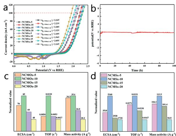
Fig. 7 (a) Polarization curves (iR-corrected) in the two-electrode configuration; (b) chronopotentiometry test of  $\text{NCMS}_{x-10}$  under overall water splitting; (c) comparison between the activities of different  $\text{NCMO}_x$  materials in 1.0 M KOH; and (d) comparison between the activities of different  $\text{NCMS}_x$  materials in 1.0 M KOH.
