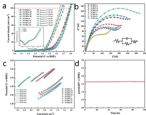
Fig. 6 (a) OER polarization curves (iR-corrected) at a scan rate of 2  $\text{mV s}^{-1}$ ; (b) OER electrical impedance maps; (c) the Tafel slopes of the materials; and (d) results of the 100 h chronopotentiometry test of  $\text{NCMS}_{x-10}$  under the OER.
