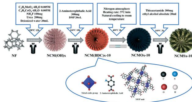
**Scheme 1** Using NiCoMn(BDC)<sub>x</sub> as a precursor, an anion exchange method was used to synthesize highly disordered NCMS<sub>x</sub> compounds.
