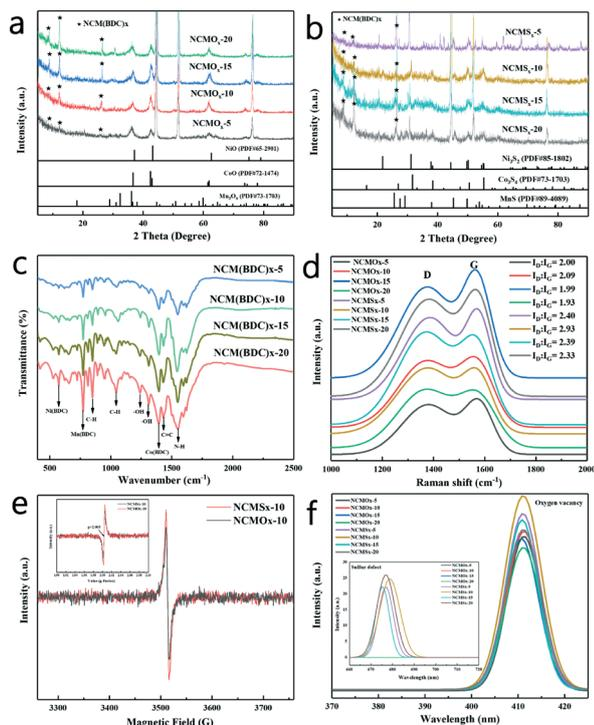
Fig. 2 (a) XRD patterns of  $\text{NCMO}_x$ ; (b) XRD patterns of  $\text{NCMS}_x$ ; (c) FTIR spectra of  $\text{NCM}(\text{BDC})_x$ ; (d) Raman spectra of  $\text{NCMO}_x$  and  $\text{NCMS}_x$ ; (e) EPR spectra of  $\text{NCMO}_{x-10}$  and  $\text{NCMS}_{x-10}$ ; and (f) PL spectra of  $\text{NCMO}_x$  and  $\text{NCMS}_x$ .
