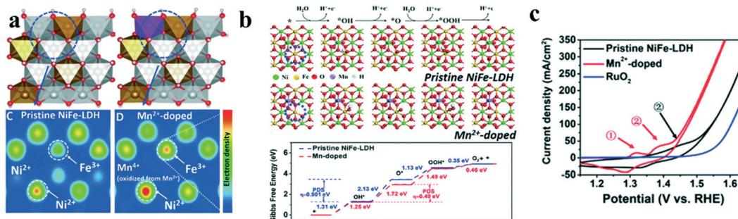
Fig. 7 Activating the basal plane of LDH for water oxidation.<sup>66</sup> (a) Schematic structure and electron density evolution based on DFT calculations, (b) four-electron mechanism of the oxygen evolution reaction and Gibbs free energy evolution based on DFT calculations, and (c) cyclic voltammetry (CV) of different catalysts for the OER tested.
