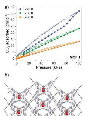
Fig. 2 (a) CO<sub>2</sub> adsorption (filled circles) and desorption (open circles) isotherms for 1 and (b) DFT-D3 optimization showing the preferential site of adsorption of CO2 in 1.
