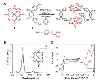
Fig. 2 (A) Synthesis of 3, Ni–Ni distance obtained by DFT (B3LYP/6-31G(d)). (B) UV/vis absorption spectrum (CH<sub>2</sub>Cl<sub>2</sub>) of 3 compared to the reference compound  ${\bf 4}$ . (C) Cyclic voltammogram of 1 mM  ${\bf 3}$  and 1 mM complex  ${\bf 4}$  in  $CH_2Cl_2$  with 0.1 M [ $^nBu_4N$ ][PF<sub>6</sub>] at 100 mV s<sup>-1</sup>
