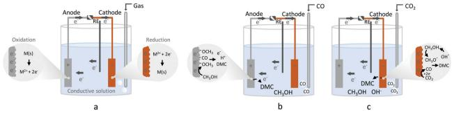
Fig. 1 Electrochemical three-electrode cells. (a) General electrochemical cell, (b) electrocatalytic synthesis of DMC with CO<sub>2</sub>, (c) electrocatalytic synthesis of DMC with CO.
