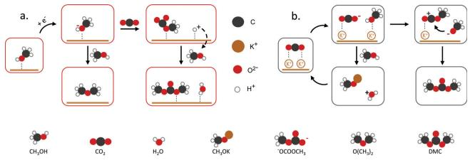
Fig. 2 Proposed mechanisms towards DMC. (a) DMC formation through methoxy and  $CO_2$ , (b)  $K^+$  interaction with  $CO_2$  to DMC. Figures adapted from ref. 25 and 33.
