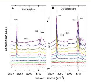
Fig. 6 FTIR spectra of an Au electrode in 0.1 M LiClO<sub>4</sub> in CH<sub>3</sub>OH with 0.1 M PhOH saturated with (A) Ar and (B) CO.55 Reprinted with permission from American Chemical Society. Copyright © 2019, American Chemical Society
