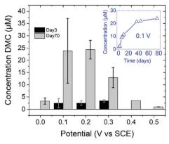
Fig. 5 DMC concentration at 3 and 70 days after electrolysis. (inset) DMC concentration change over time since the day of electrolysis, shown for 0.1 V vs. SCE.<sup>38</sup> Reprinted with permission from American Chemical Society. Copyright © 2019, American Chemical Society.
