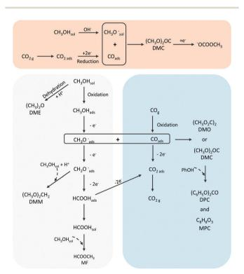
Fig. 7 Suggested reaction pathways and intermediates from CO<sub>2</sub> or CO and CH<sub>3</sub>OH.
