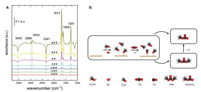
Fig. 3 (a) FTIR spectrum of CO<sub>2</sub> reduction in CH<sub>3</sub>OH on a Cu electrode at potentials between -1.2 and -2.4 V vs. Ag/AgCl.<sup>10</sup> (Reprinted with permission from American Chemical Society. Copyright©2019, American Chemical Society.) (b) Proposed reaction mechanism that involves the electrochemical reduction of CO<sub>2</sub> to CO with a simultaneous activation of CH<sub>3</sub>OH. Scheme adapted from ref. 10.
