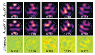
Randomly chosen examples of the MLP-predicted profile  $A_{pred}$ , the corresponding true profile AFDTD, and the difference between the two profiles (difference). The integrated absorption ( $\lambda$  = 600 nm) for each profile is included at the bottom of each panel. The  $\sigma_{pp}$  metric for each pair is included at the bottom of the difference panel
