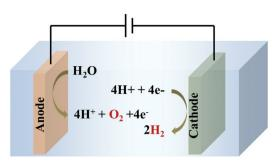
Scheme 1 Electrochemical water splitting to generate  $O_2$  and  $H_2$  by simultaneous water oxidation (at the anode) and water reduction (at the cathode), respectively.
