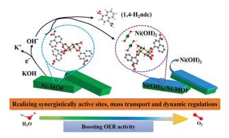
Scheme 3 A schematic representation of the transformation of Ni-MOF to Ni(OH)2/Ni-MOF heterostructure and the synergistic catalytic OER process by Ni(OH)<sub>2</sub>/Ni-MOF. Adapted with permission from (ref. 81). Copyright (2020) American Chemical Society
