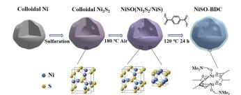
Scheme 5 Schematic illustration of the preparation of Ni-BDC-modified  $Ni_3S_2/NiS$  (NiSO-BDC) hollow nanoparticles. Reprinted with permission from (ref. 126). Copyright (2019) American Chemical Society.
