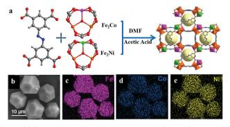
Fig. 1 (a) Schematic diagram of the synthesis of PCN-Fe<sub>2</sub>Co-Fe<sub>2</sub>Ni. (b) Scanning electron microscopy (SEM) image and (c-e) corresponding elemental (Fe, Co and Ni) mapping images for PCN-Fe<sub>2</sub>Co-Fe<sub>2</sub>Ni. Adapted with permission from (ref. 82). Copyright (2019) American
