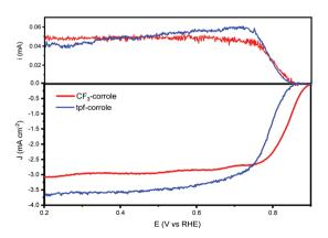
Fig. 2 RRDE of CF<sub>3</sub>-corrole and tpf-corrole in 0.1 M KOH @ 900 rpm.
