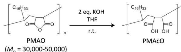
Scheme 1 Hydrolysis reaction of PMAO to form PMAcO.
