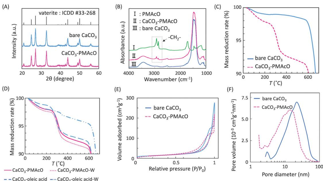
Fig. 3 Physical properties of bare  $\text{CaCO}_3$  and  $\text{CaCO}_3$ -PMAcO microspheres: (A) XRD spectra, (B) FT-IR spectra, (C) TG curves, (D) TG curves of  $\text{CaCO}_3$ -PMAcO and  $\text{CaCO}_3$ -oleic acid before and after washing; “-W” indicates samples after washing, (E)  $\text{N}_2$  adsorption-desorption isotherms, and (F) pore size distributions.
