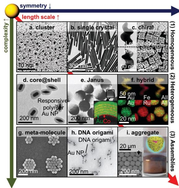
Fig. 2 Hybrid Au nanoparticles. (a) Clusters,<sup>47</sup> (b) single crystal nanowire,<sup>52</sup> (c) chiral NPs,<sup>31,45</sup> (d) core–shell NPs,<sup>27</sup> (e) Janus NPs,<sup>23</sup> (f) alloyed NPs,<sup>142,174</sup> (g) plasmonic meta-molecules,<sup>175</sup> (h) DNA-origami templated assemblies,<sup>25</sup> (i) large-scale assemblies of NPs.<sup>99,176</sup> Adapted by permission from the corresponding references. Copyright American Chemical Society, Springer Nature, Wiley-VCH.
