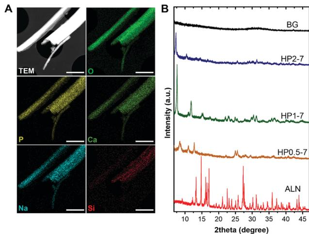
Fig. 3 (A) Scanning TEM image and EDX elemental maps of single HP1-7 particles. (B) Powder XRD spectra of different particle types. Scale bars in images correspond to 1  $\mu\text{m}$ .
