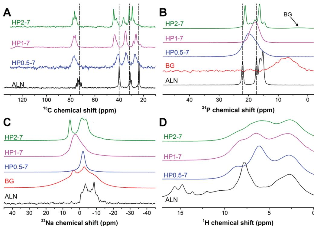
Fig. 4 Solid-state CP-MAS NMR spectra of different types of hybrid particles.
