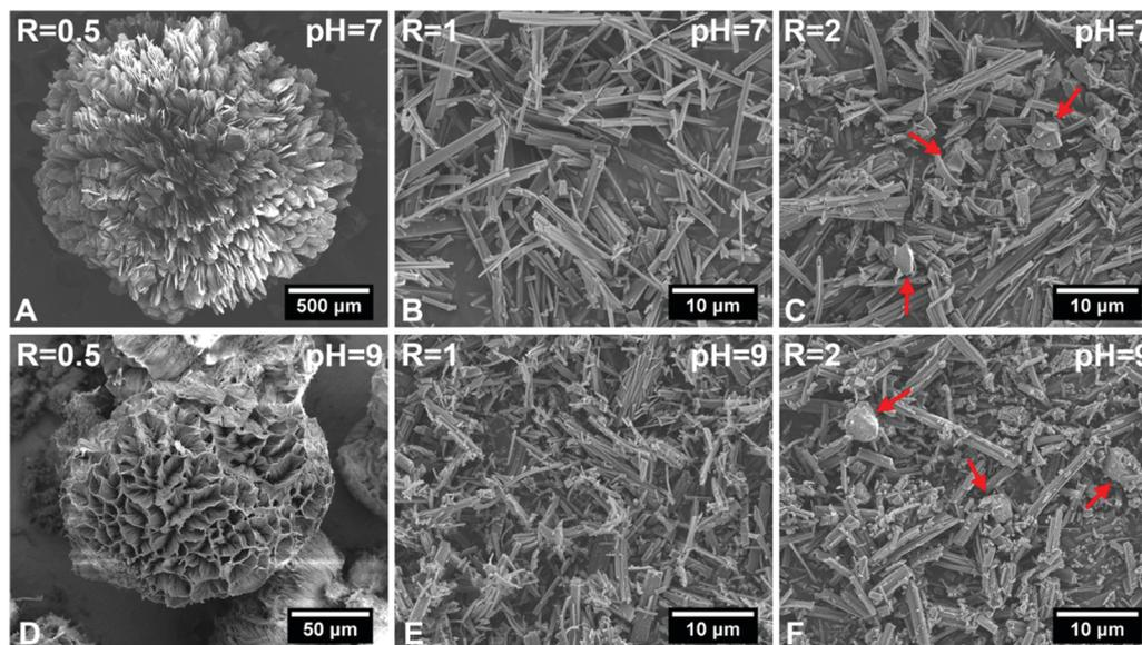
Fig. 1 Scanning electron micrographs of hybrid particles precipitated at different  $\text{Ca}_{\text{BG}}/\text{ALN}$  ratios ( $R$ ) and pH values after 3 days of incubation at 37 °C. Red arrows indicate bioactive glass residues.
