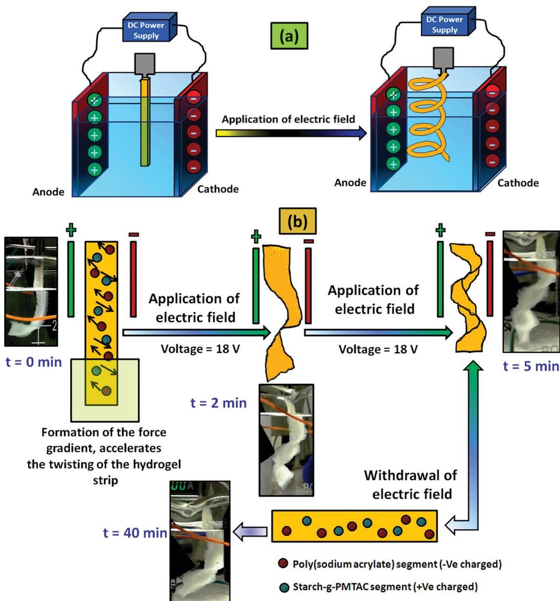
Fig. 10 (a) Schematic representation of the actuation in the polyelectrolyte composite hydrogel (PSAS<sub>50</sub>C<sub>5</sub>) system in the presence of an electric field and (b) behaviour of the composite hydrogel (PSAS<sub>50</sub>C<sub>5</sub>) system with the time of electric field application.
