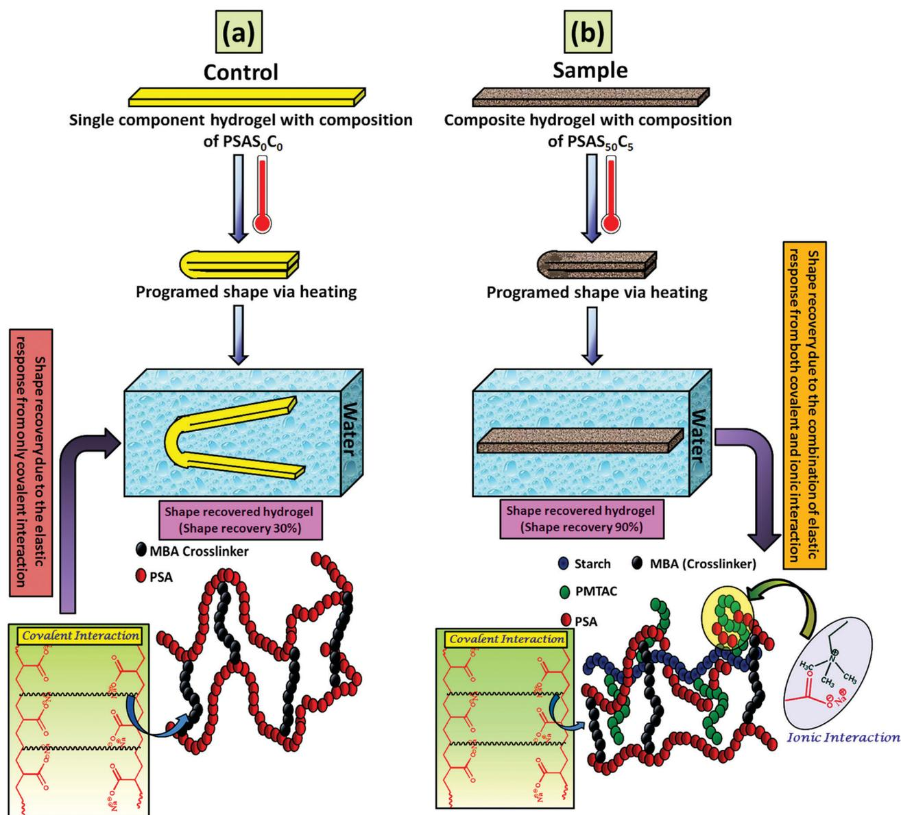
**Scheme 2** Schematic representation of the shape memory effect shown by the hydrogel having a composition of (a)  $\text{PSAS}_0\text{C}_0$  (control) and (b)  $\text{PSAS}_{50}\text{C}_5$  (sample) after subsequent treatment with heat followed by water and the respective mechanisms acting behind the shape memory effect.
