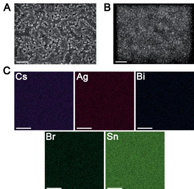
Fig. 5 SEM images of thin films of (A) **1** and (B) **1:Sn** (4 atom% Sn). (C) Elemental mapping on a thin film of **1:Sn** (4 atom% Sn) using EDX. The scale bars in (A) and (B) are 500 nm and the scale bars in (C) are 2  $\mu\text{m}$ .
