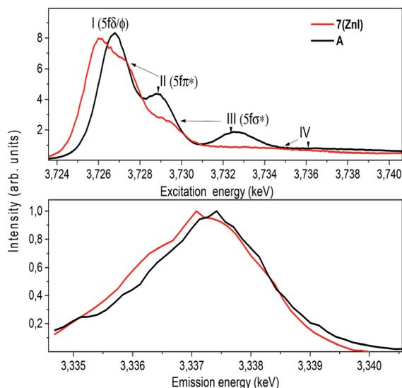
Fig. 10 Uranium  $M_4$  edge HR-XANES (top) and resonant X-ray emission (RXES) (bottom) spectra of complexes 7 (ZnI) and A. The RXES are measured at excitation energies corresponding to the maximum intensity of the first peak (I) of the respective HR-XANES spectrum.
