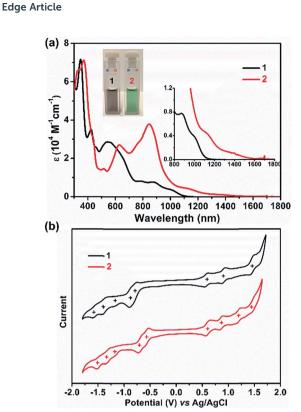
Fig. 4 (a) UV/Vis absorption of 1 and 2 recorded in dry DCM. Insets give a magnified view and the photos of their DCM solutions. (b) Cyclic voltammograms of 1 and 2 in a solution of Bu<sub>4</sub>NPF<sub>6</sub> (0.1 M) in DCM with a scan rate of 50 mV s $^{-1}$  at room temperature.
