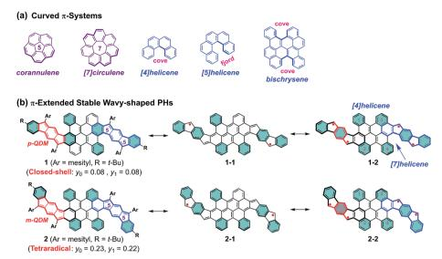
Fig. 1 (a) Representative curved  $\pi$ -systems. (b) The resonance structures of  $\pi$ -extended stable wave-shaped PHs 1 and 2 reported in this work  $(p-QDM \text{ and } m-QDM \text{ units are highlighted in red color; the flanked indeno[1,2-b]fluorene (IF1) and indeno[2,1-b]fluorene (IF2) in 1 and 2 are$ highlighted in blue color). The substituents are omitted in the resonance structures for clarity and the benzene rings in cyan color denote Clar's aromatic sextet rings.
