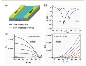
Fig. 5 Solution-processed thin-film transistors of 2. (a) Schematic illustration of the transistor. (b) Transfer characteristics for an ambipolar transistor based on the spin-coated film of 2. (c) Transistor output curves of the spin-coated film of 2.
