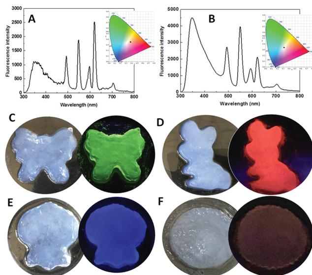
Fig. 6 Emission profiles of Eu–Tb–Dy MOF gels under the single-wavelength excitation at 275 nm with the Eu/Dy/Tb ratios of (A) 1 : 1 : 1 and (B) 1 : 1 : 2. Photographs of (C) Tb–Dy, (D) Eu–Tb, (E) Eu–Dy, and (F) Eu–Tb–Dy MOF gels with mixed-metal ratios of 1 : 1 or 1 : 1 : 1 under sunlight (left) and excitation at 275 nm (right).
